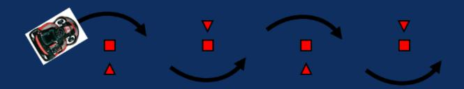
The Swiss slalom consists of several challenges made up of individually placed cones arranged in a line which must be driven around on alternating sides.
