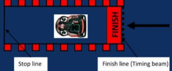
Tip: You can have the Start line after Finish/Stop line in order to minimize downtime to turn and roll the kart to Start line. Make sure you leave a safe distance between Stop line and Start line
