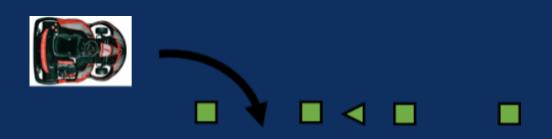
A change over gate consists of two cone gates which must be passed in succession. The cones of a changeover gate are placed in a straight line. The distance between the gates must be at least 1.5m and not exceed 4m.
