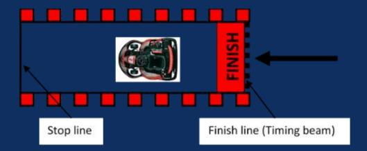
The Finish sensor barrier must be located immediately before the first cones of the finish lane. The cones in the finish lane are scored individually.
